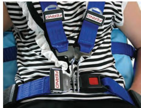
Fig 8 Buckle through Slots
