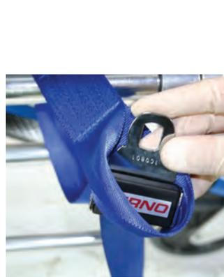
Fig 6 Feed Buckle through loop
