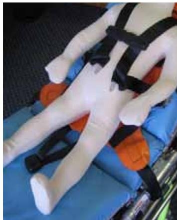
Fig 7: Shoulder straps in place for crotch strap buckle
