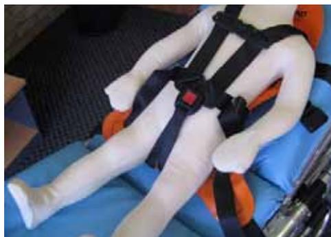
Fig 8: Shoulder and crotch strap fitted
