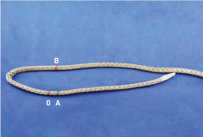
A “Locked Brummell Splice” may be made, using only one end of the rope, in most Hollow Braid ropes.
