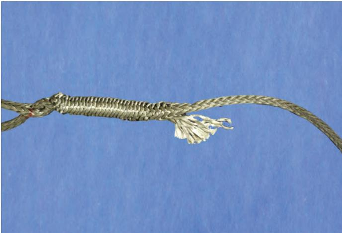
**Step #14** – Remove fid and tape, pull End 1 until 1/2 of a full fid length is exposed at the exit point. Fan all the ends out and cut ends on an angle to provide a smooth taper.
