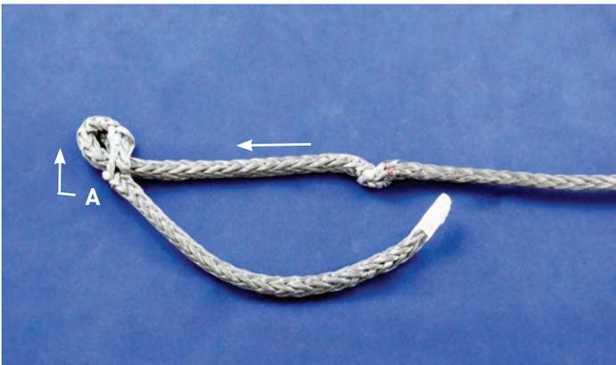
**Step #8** – Now Un - Roll point A. working rope up and through point A. in direction shown.
