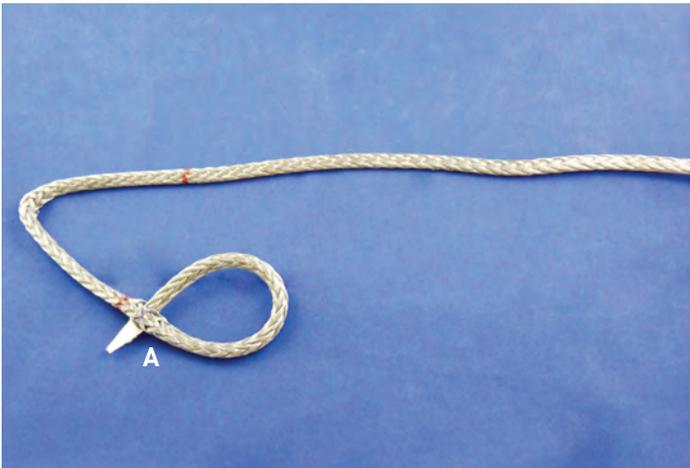
**Step #2** – Attach the end to a fid and pass them through the center of rope at Mark A.
