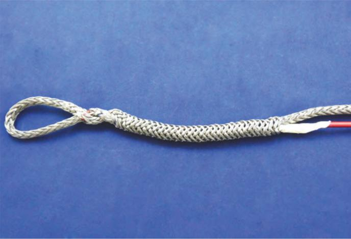
**Step #13** – Finally, bury tail into standing end. Attached the fid to the tail of the rope. On the standing part of the rope, measure one rope diameter below where the tail exits the standing part of the rope, this will be the entry point.
