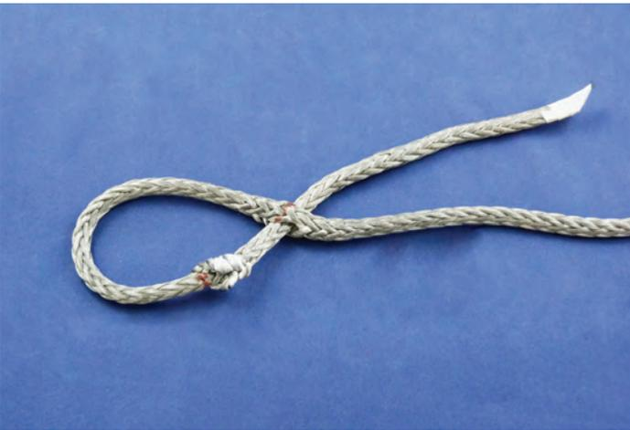
**Step #5** - Now pass end through center of rope at Mark B.
