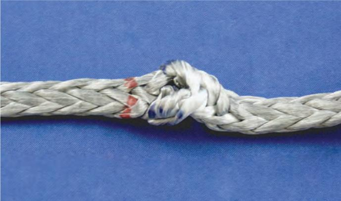
**Step #4** - Pull end hard to roll "inside-out" at Mark A.
