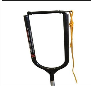
The large Carbon Fibre Line Hook attaches a line to a fixed point at height or across water. Its opening width measures 165 mm. It can be used, for example, to secure a line to a submerged vehicle.
