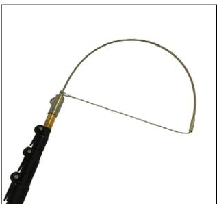
The Pro Snare is a spring loaded device. The loop is placed over the target. A light tug to the pole releases the snare thus locking it on to the target.
