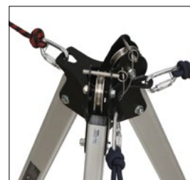
The advanced IndustriPOD+ has a one-piece fabricated steel head with two integrated 70mm sheave pulleys and three 360kg stabilisation anchor points
